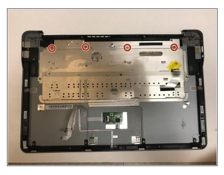
Remove the four Phillips #00 screws that hold the keyboard to the laptop case.
