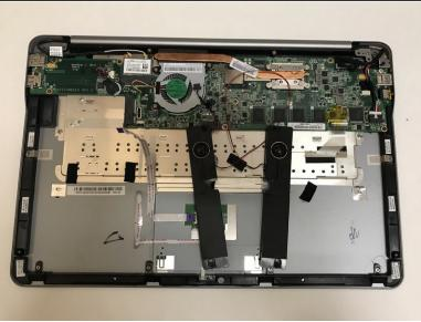
Pull off the black strips of tape from the speaker wires and remove the speakers from the laptop.
