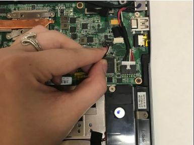
Unplug the wire connecting the speakers to the motherboard.
