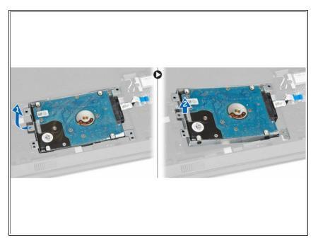
• Lift the hard drive to remove it from the computer.
