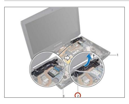
Slide and lift the routing guides off the computer base.
