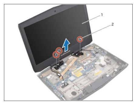
Place the **NEW** display assembly in position and replace the screws, on the display hinges, that secure the display assembly to the computer base.
