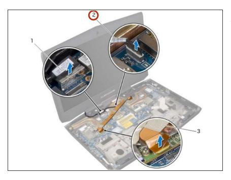
Disconnect the LED-logo board cable from its connector on the system board.
