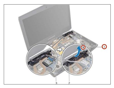
Remove the screw that secures the routing guides to the computer base.
