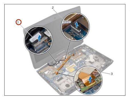
Pull the pull-tab to disconnect the display cable from its connector on the system board.
