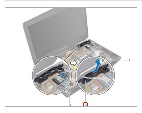
Place the routing guides on the computer base and replace the screw that secures the routing guides to the computer base.
