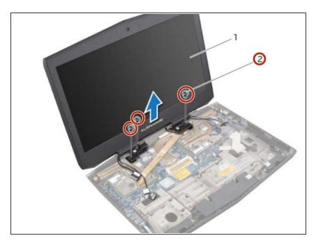
Remove the screws, on the display hinges, that secure the display assembly to the computer base.
