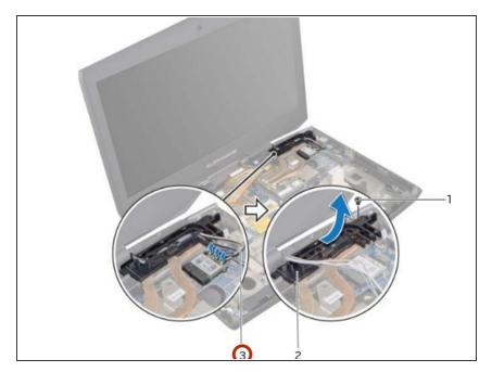
Route the Mini-Card antenna cables through the routing guides on the computer base.
