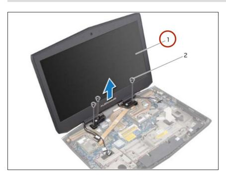
Move the display to a perpendicular position to the computer base, and then lift the display assembly off the computer.
