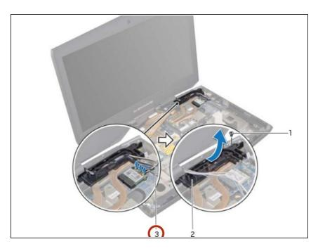
Note the routing of the antenna cables, and then remove the cables from the routing guides on the computer base.
