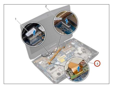
Disconnect the video-card connector cable from its connector on the system board.
