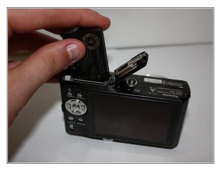
Remove the battery and the SD Card.
