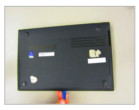
Slide the plastic the spudger along the edge of the device to separate the keyboard tray.
