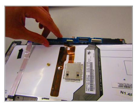
Gently wiggle and lift the Push Button board from the keyboard tray.
