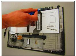
• Unlock and remove the 3 ribbon cables along the top of the keyboard tray.
