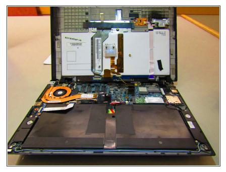
Flip the device over and open it to lift the keyboard tray from the body of the device.
