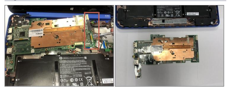
• Now, gently pry up on the right side of the motherboard with the spudger and then lift the motherboard out.
