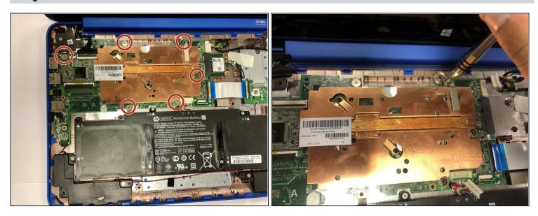
• Using a Phillips #0 screwdriver, remove the six screws holding the motherboard down.
