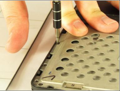
• Remove the thirteen 2.85mm Phillips #00 screws from the screen.
