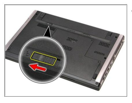
Slide the other battery release latch to the unlock position.
