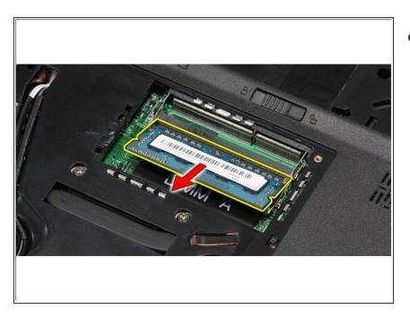
Remove the memory module from its connector on the system board.
