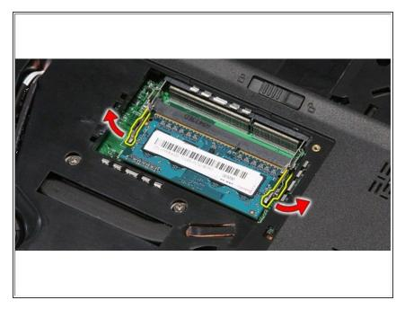
Push apart the memory retention clips to release the memory module.
