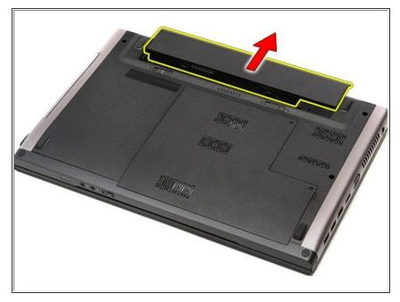
Slide the battery and remove it from the computer.
