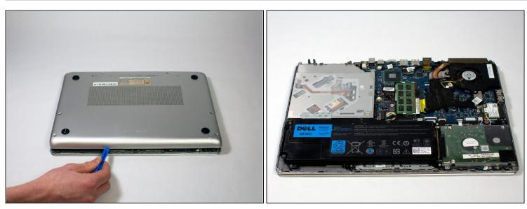
• Using the plastic opening tool, pry up the back cover.
