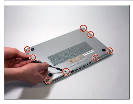
Remove the back cover of the laptop by unscrewing eight 3.5mm screws using a Phillips #0 screwdriver.
