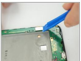
Use the Plastic Opening tools to gently dislodge the two connection on the top and bottom right of the phone from the inside of the phone.
