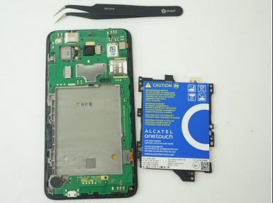
• Use a pair of tweezers to pull the battery connector from its port.
