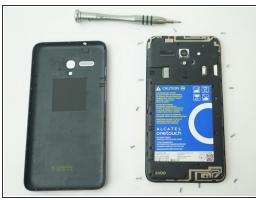
Remove 13 1mm JIS screws with JIS #000 Screwdriver.
