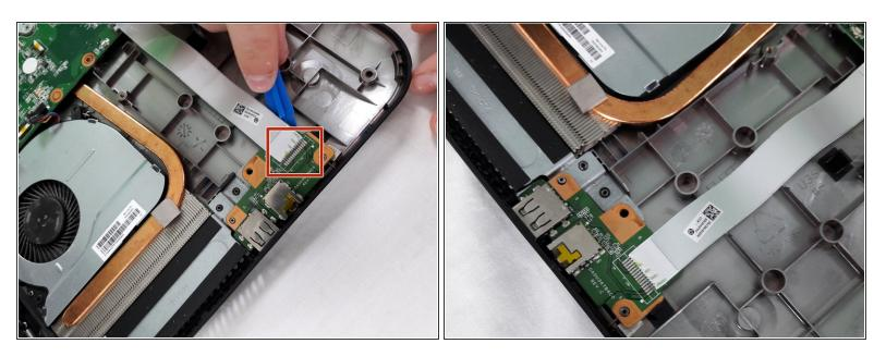
Disconnect motherboard cable from left side USB and jacks
