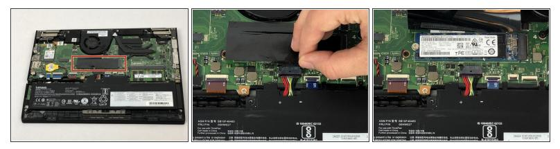
• Pull back the plastic heat shield over the hard drive without tearing or completely removing it.
