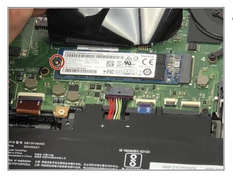
Using a Phillips screwdriver, remove the PH1 Phillips fastener and set it aside.
