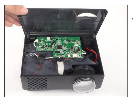
• Flip the projector over and then remove the cover by lifting it up.
