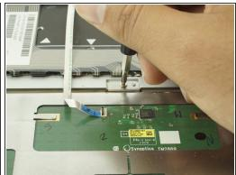
Using the PH00 Screwdriver, remove the five 2.0 mm screws indicated in the picture.
