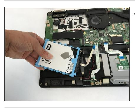
Lift the hard drive up and out of the laptop.
