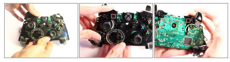
Align the replacement bumper onto the pegs, push gently and click into place.
