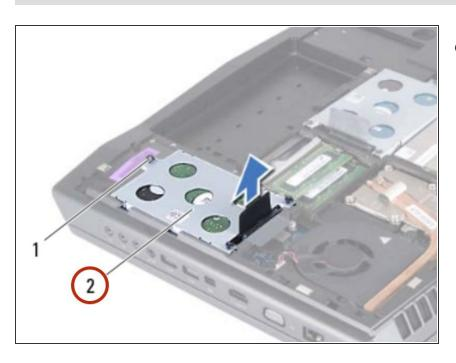
Using the pull-tab, lift the hard-drive assembly to disconnect it from the connector on the system board.
