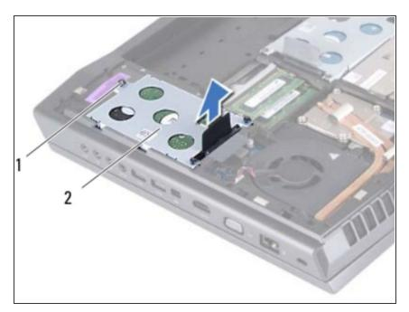
Tighten the three captive screws that secure the hard-drive assembly to the computer base.
