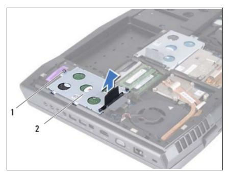
Align the connector on the hard drive with the connector on the system board and press the hard drive until it is fully seated.
