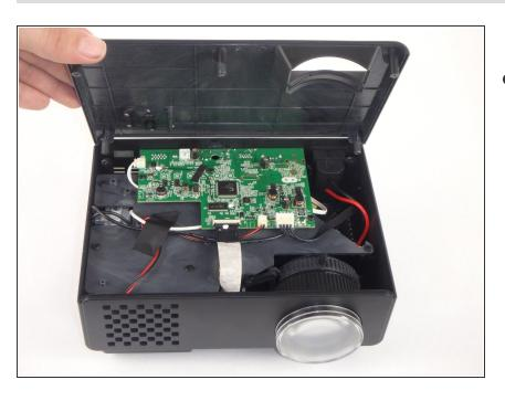
Flip the projector over and then remove the cover by lifting it up.
