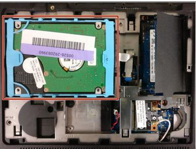
Remove the small panel on the back by prying it off. This should reveal the hard drive.
