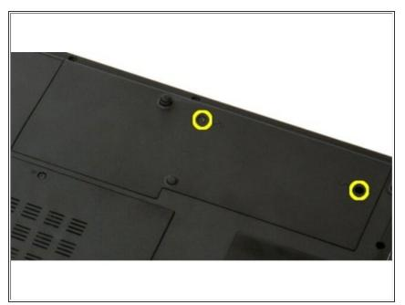
• Remove the two screws that secure the hard drive and mini-card access panel to the computer.
