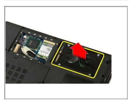
• Lift and remove the hard drive from the computer.
