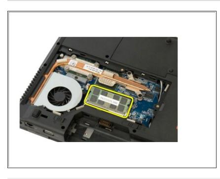
Remove the memory module from the socket
