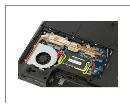
Using your fingertips, carefully spread apart the securing clips on each end of the memory module
