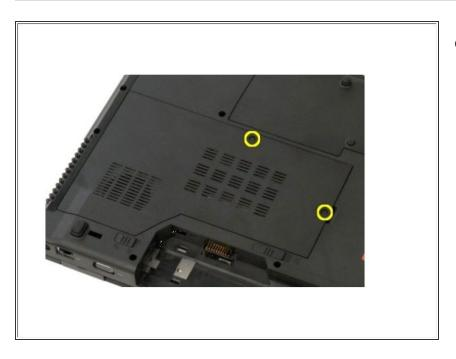
Loosen the two captive screws on the access panel.
