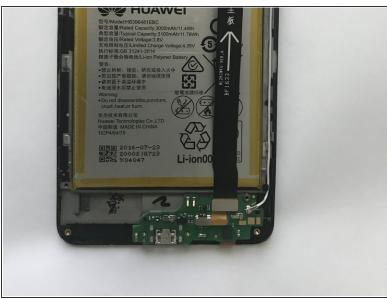
Remove the six 1.5mm Phillips #000 screws from the bottom of the phone.
