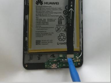
Use a plastic opening tool to disconnect the white and black antenna cables from the daughterboard.
