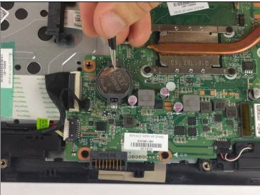
• Use long nose <u>tweezers</u> to reach under battery and lift up.
