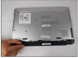
• Slide the battery release switch to the right until the battery pops out.
