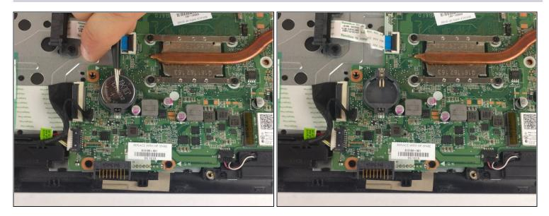
• Lift up until battery pops out, remove battery
