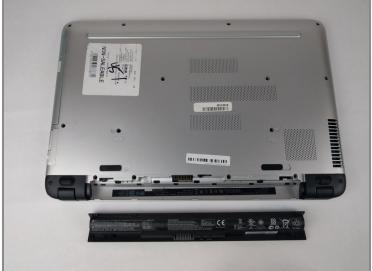
• Grabbing the top edge of the battery, rotate it toward you and then lift upward to relieve the battery from its slot.
