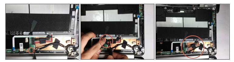
• Disconnect the DC jack cable and the battery cable from the motherboard using tweezers, the pointed end of a plastic spudger, or by simply pulling the cables apart from the motherboard with your fingers.
