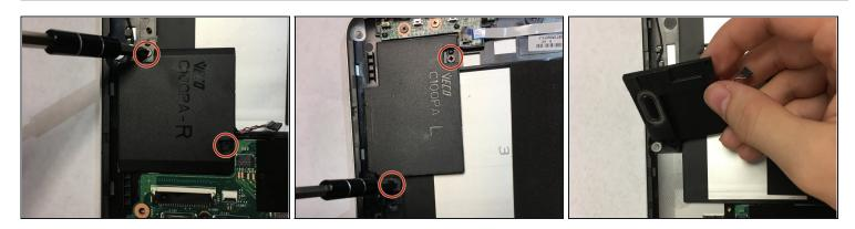
• Remove the four 4.2mm speaker screws, then remove the two speakers using a Phillips #0 screwdriver.
