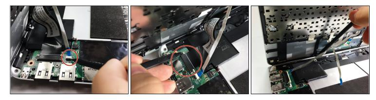
• Disconnect the touchpad cable and the keyboard cable on the palm rest assembly from the motherboard using the pointed end of a plastic spudger.
