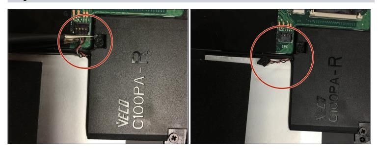
• Disconnect the speaker cable from the motherboard using tweezers or the pointed end of a plastic spudger.
