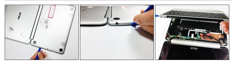
• Pry the palm rest assembly apart from the bottom cover using a spudger. This step may require extra power. Once the palm rest has been separated from the bottom cover, pull it away from the screen, rather than away from yourself.
