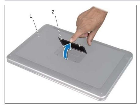
• After turning off the computer, turn over the laptop and lift up the system badge (#2).
