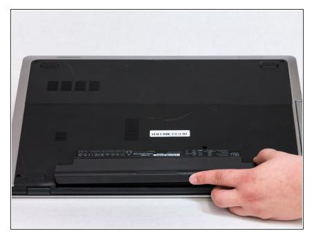
• Lift the battery up and out of the laptop battery socket.
