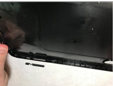
Remove the old button and replace it with the new one.
