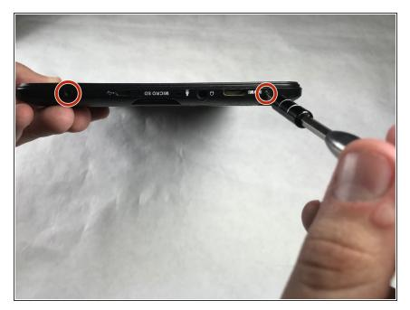
Remove the two 3.2 mm PH000 screws near the charging port.
