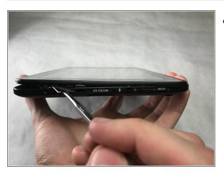
Pry the back cover from the device along bottom edge.
