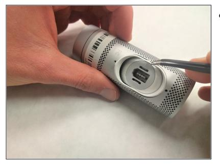
• Insert the <u>tweezers</u> into the crevice of the ball and socket joint, and prop up the tabs to remove the white ring from the body.
