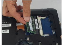
Press down on the tabs on both sides of the RAM to release, then pull away from the mount to remove.
