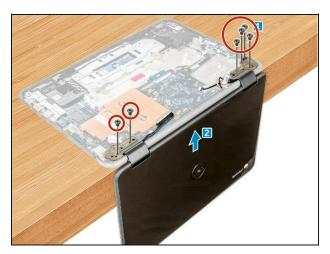
Replace the screws that secure the display hinges to the palm-rest assembly.
