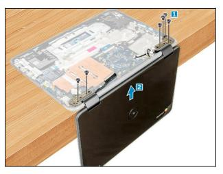
Place the display assembly to align with the screw holders on the computer.
