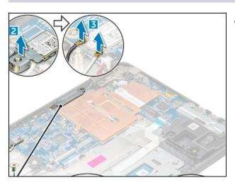
Connect the WLAN cables.
