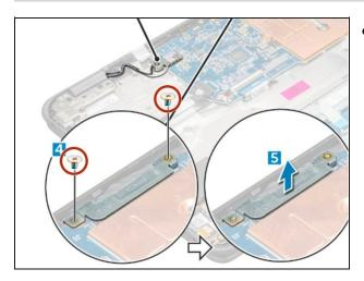
Place the metal bracket over the (display cable) connector, and tighten the M2.0x3.0 screws to secure the display cable to the computer.
