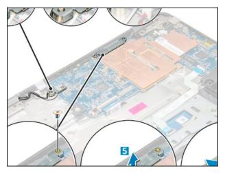
Place the metal bracket, and tighten the M2.0x3.0 screw to the WLAN cable on the system board.
