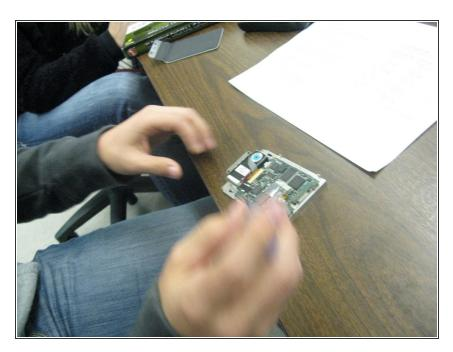
Unscrew the two screws that hold the scrollwheel to the motherboard.
