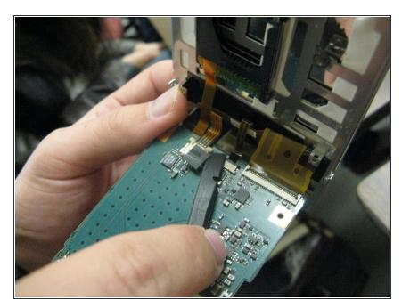
Remove ribbons that connect the screen to the motherboard and remove battery
