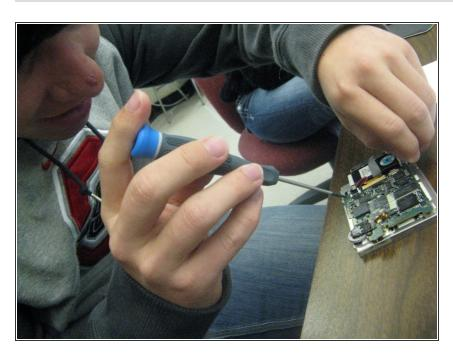
On the back of motherboard, unscrew the 5 screws on the back
