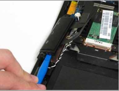
Find an opening on the side of the port and pry the USB and AUX port out of the laptop with the prying tool.
