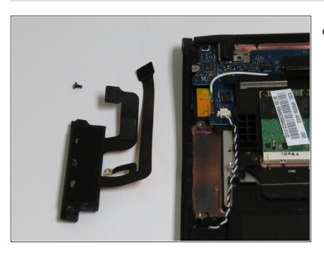
Remove and place the port outside of the laptop. You are free to install your new USB and HDMI ports.
