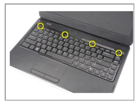
Pry up to release the top four snaps securing the keyboard to the computer.
