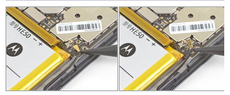
• Use the point of a spudger to pry up and disconnect the antenna cable from its motherboard socket.
