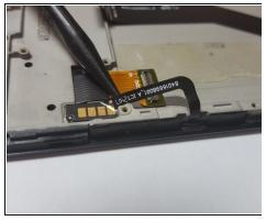
• Use the <u>Precision Tweezer</u> to detach the <u>Power and Volume Buttons Flex</u>. Start at the lip of the phone, as seen in Image 2, and lift up. Slide the precision tweezers under the power and volume buttons flex until you reach the gold plated section, detaching it from the phone.
