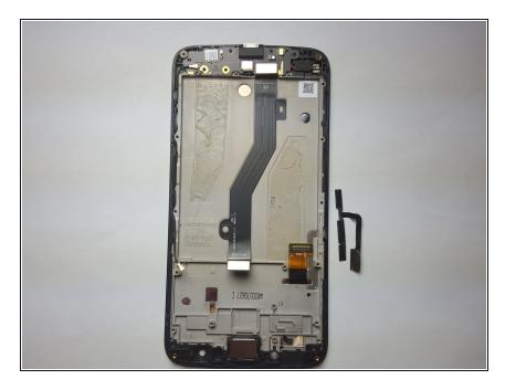
This is the result of removing the volume and power buttons flex from the phone.
