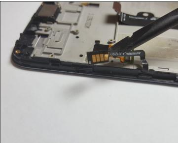
• Use the <u>Plastic Spudger</u> to finish lifting the volume and power buttons flex from the base of the phone.
