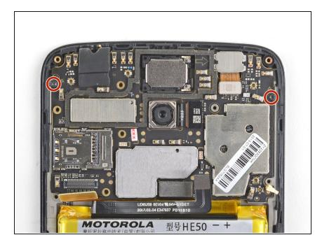
Remove the two black 3.2 mm long T3 screws securing the motherboard.
