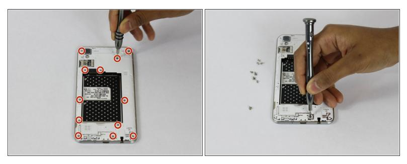
• Remove the twelve 2mm JIS #00 screws from the mid-frame.
