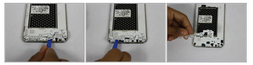
• Using a plastic opening tool, remove the antenna extender from the mid-frame.
