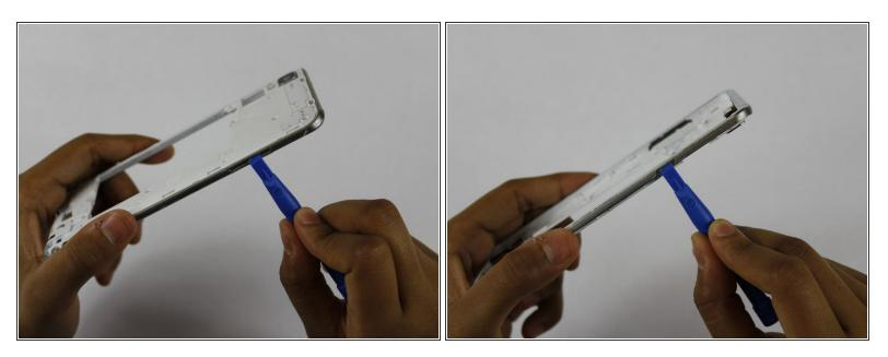
• Use a plastic opening tool to remove the buttons by pushing them in until they pop through.
