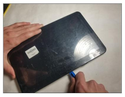
Insert the plastic opening tool between the white back cover and black front over.
