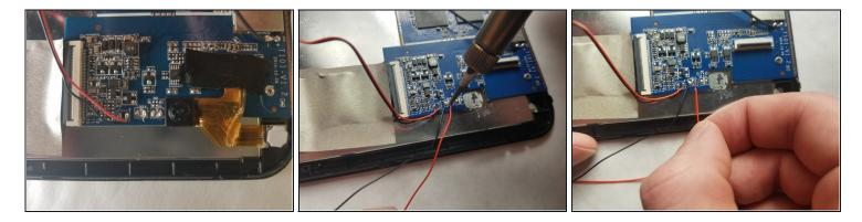
• Desolder the red and black wires connecting each speaker to the motherboard.
