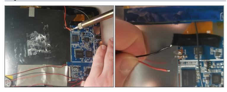
• <u>Desolder</u> the red and black wires connecting the battery to the motherboard and remove the battery.
