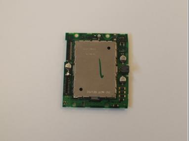
Now it's time to replace the sound board! Unhook your old Sound board from your Docking cradle assembly. Now that the old Sound board is uninstalled, take your new one and hook it up to the Docking cradle assembly with the 24FF cable. It will be the only cable that is there.
