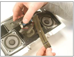
Now you are ready to unscrew the Amplifier board and lift to create slack in the 20C Flex cable.
