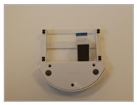
Hook the Flex cable from the Amplifier board to your Sound Board. Once the connection is solid and secure, Install Docking cradle assembly back into its spacers slots.
