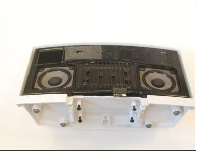
• In order to reach the Sound Board to fix the audio problem on your Bose SoundDock you must first take the bottom plate off using a standard Phillips Screwdriver.
