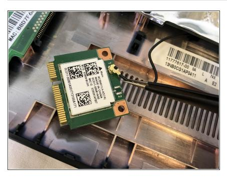
Disconnect the antenna cable from the Wi-Fi chip.
