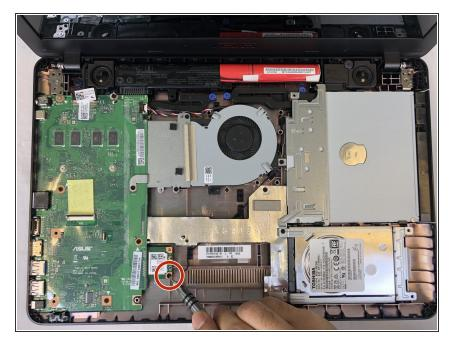
Remove the 6mm Phillips #0 screw from the Wi-Fi card.
