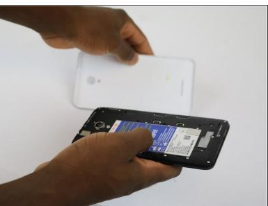
Remove the back cover by sliding your fingernail in the grove around the edge of the phone and prying it off.
