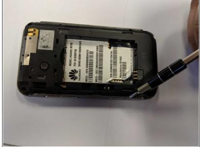
Using the T5 Torx screwdriver, remove the six 6mm screws.
