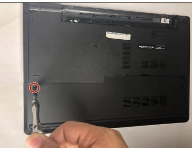
Use a Phillips #1 screwdriver to remove the two 2.5x8mm screws on the back panel.
