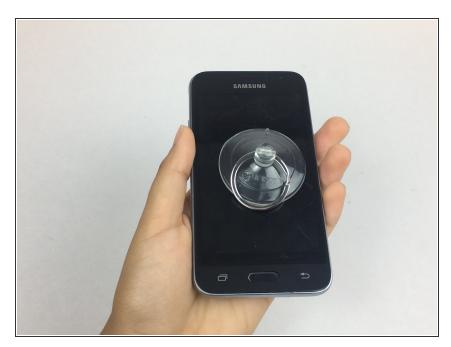
Attach a small suction cup to the lower half of the glass screen.
