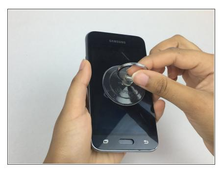
Apply pressure to the middle section of the screen while pulling up the lower edge by pivoting your wrist.
