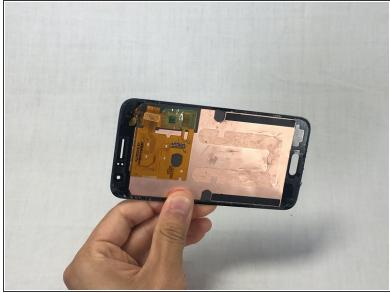
Pull the rear panel up and away to completely separate it.
