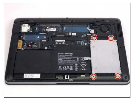
Remove the hard drive by unscrewing the four 8mm screws with the T7 philip's head.
