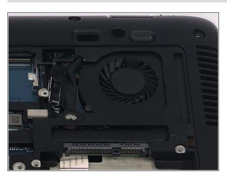
Use an opening tool to pry up the ribbon connector to disconnect.
