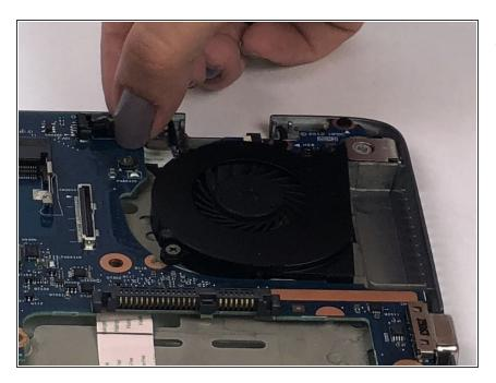
Unplug fan cable by pulling away from its connector.
