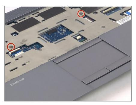
Remove the two 4mm screws centered notated by the keyboard logo using the J00 tip.
