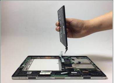
Carefully remove the battery from the device by lifting it up.
