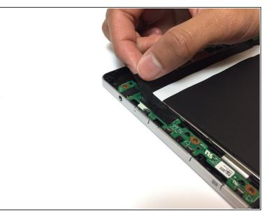
Remove the piece of black, thin tape that is attached to the circuit board closest to the power button.
