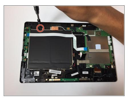
Using the Phillips #000 screwdriver, remove the 3 mm screw that is holding the battery in place.
