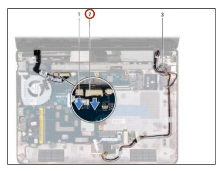
Disconnect the display cable and the camera cable from the system board connectors.
