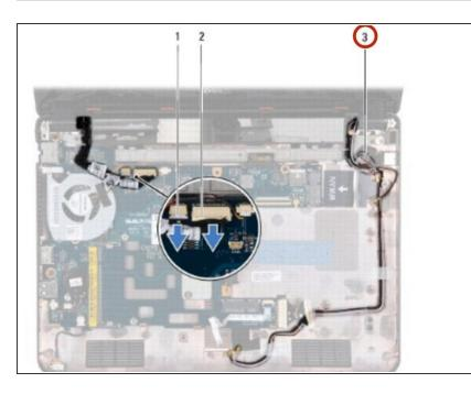
• Route the Mini-Card antenna cables through the routing guides.
