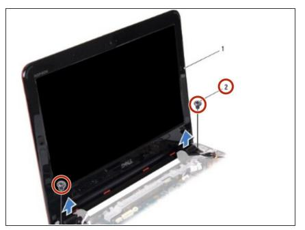
Remove the two screws (one on each side) that secure the display assembly to the computer base.
