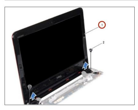
• Lift the display assembly off the computer.
