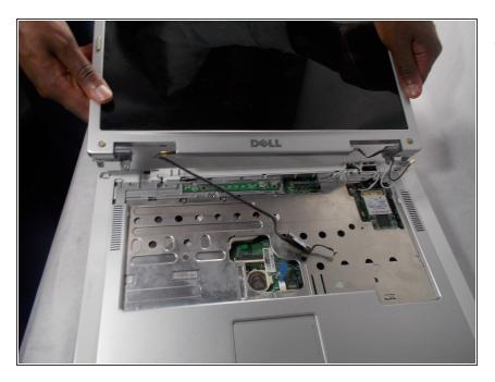
• Remove the display from the rest of the device.
