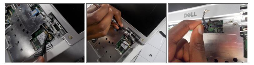
• Disconnect the antenna cables from the Mini-Card.
