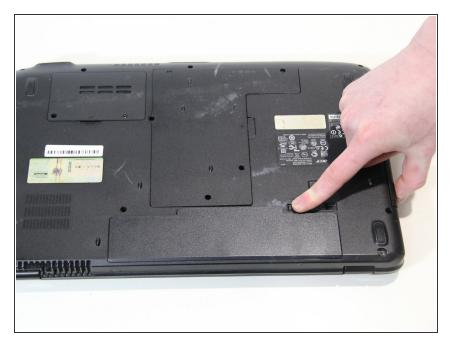
Slide the release latch to the left to release the battery from the PC.
