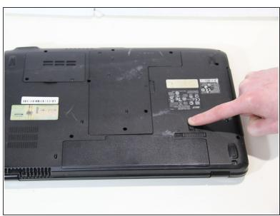
Unlock the battery by flipping a switch near the release latch.
