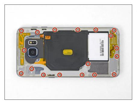
Remove eighteen 3.2 mm screws from the midframe.
