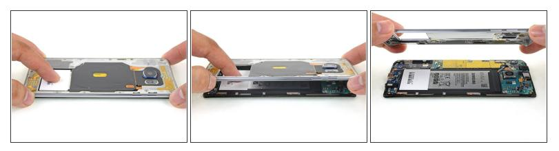
Press down on the back of the battery while you lift up on the edges of the midframe to separate the midframe from the rest of the phone.
