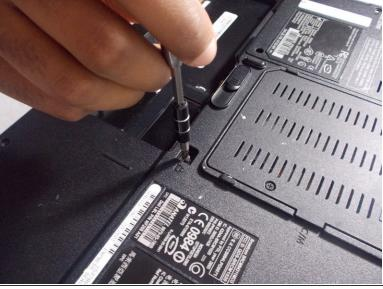
Remove the JIS #1 8mm screw from above the upper right corner of where the battery was.
